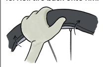
Use the heel of your hand to work the tire back on the rim, starting at the valve. If you use levers for this, careful not to puncture the tube!
